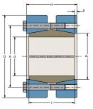
Note: Shaft engagement equal for both ends with gap not exceeding 5% of shaft diameter.
